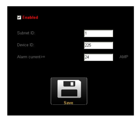
In the Smart G4 HAC software for Windows, just go to settings -> power meter -> Enter the Device ID of your power meter Module. And press save. It will do the reading for you.
