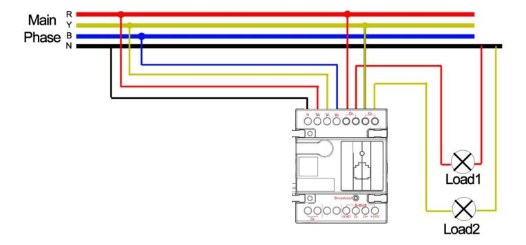
Above is an example of connecting two different loads on different phases to the Smart G4 power meter.
